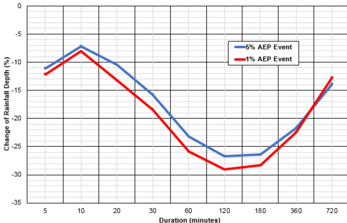
Diagram 2 indicates that design rainfalls have decreased by up to 30% for durations between 40 minutes and 4 hours using ARR2019. For 360 to 720 minutes the reduction ranges from 25% to
